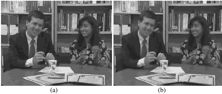
Fig. 7. Performance of the deblocking filter for a highly compressed image (QP=38) (a) Reconstructed Paris Image without Filtering. (b) Reconstructed Paris Image with Filtering
