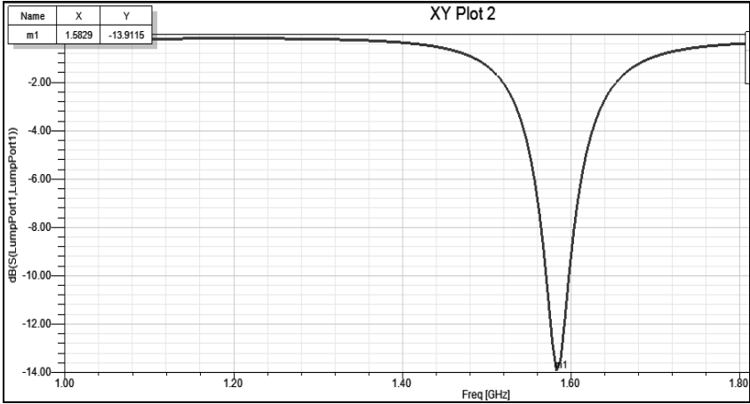
Fig. 2. Reflexion coefficient ( S_{11} ) for single element
