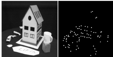
Fig. 2. Illustration of the Harris-Stephens procedure
