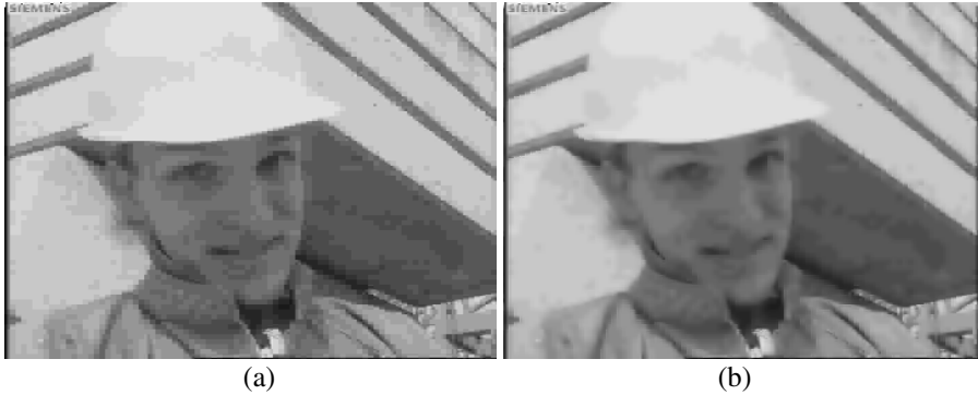
Fig. 6. Performance of the deblocking filter for a highly compressed image (QP=38) (a) Reconstructed Foreman Image without Filtering. (b) Reconstructed Foreman Image with Filtering
