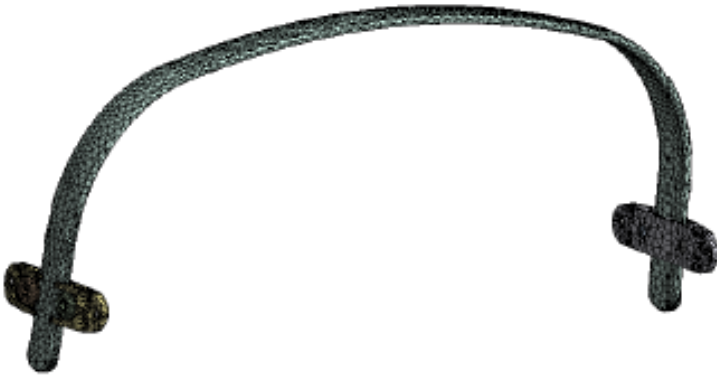
Fig. 2. Discrete model of the system. Finite element - SOLID187
