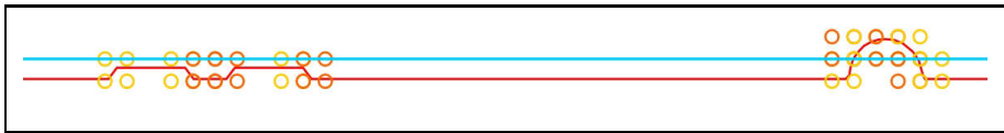
Fig. 2. An example for the COLLINEAR MERGE step. Circles highlight approximation points, the polyline represents (part of) the input polygon P , and the long straight line represents an approximation segment computed by the COLLINEAR MERGE step.
