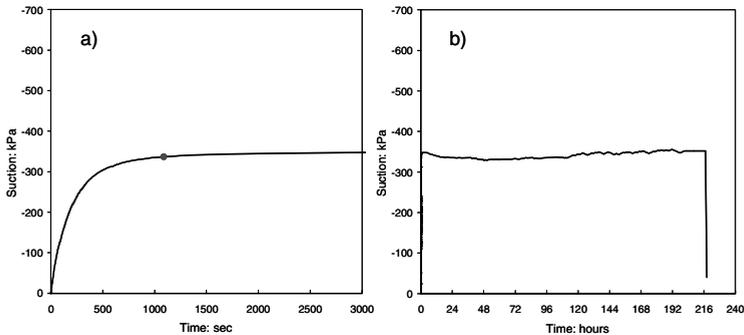
**Fig. 6.** Long time suction measurement on soil sample.
