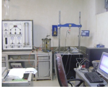
Fig. 2. The test set up for unsaturated soil.
