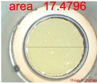
Fig. 1. Sample shrinkage after application of suction.
