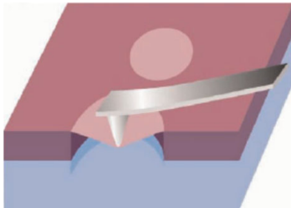
Fig. 4.4 Measurement of graphene elastic modulus: Schematic of indentation on suspended graphene (Figure/Caption Reprinted (Adapted) from [36], Copyright (2009) WILEY-VCH Verlag GmbH & Co. KGaA, Weinheim)
