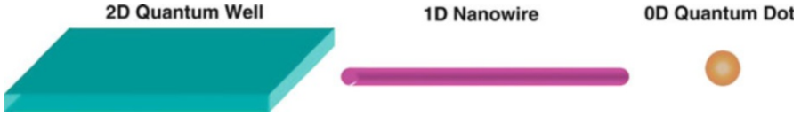
Fig. 2.1 Schematics of nanostructures of 2D quantum well, 1D nanowire, and 0D quantum dot
