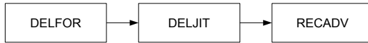
Fig. 6. Model of a fictional supply chain management process consisting of delivery forecasts, just-in-time delivery requests and receiving advices
