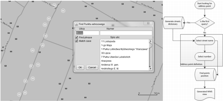
Fig. 6. A search of an address point on the base of a street name and a number
