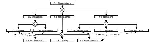
Fig. 1. Component model for a photovoltaics installation
