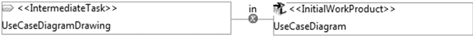
Fig. 9. An example of a validation error in the constraint on the relation between intermediate tasks and work products
