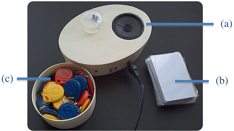
Fig. 1. (a) TV-Companion device (b+c) with RFID tokens. The device's electronics components comprise an Arduino microprocessor board, a RFID reader module, infrared TV remote control, a module for playing back wave recordings and speakers.
