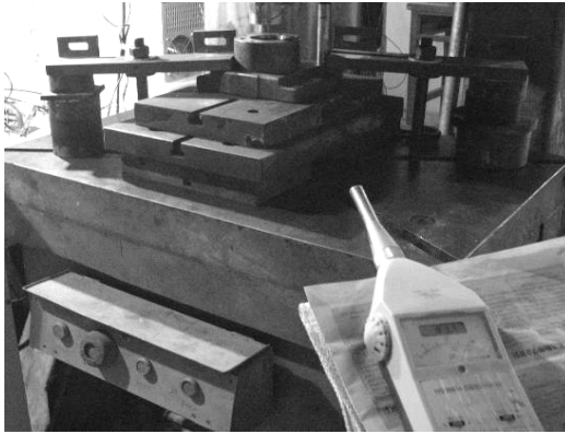
Fig. 7. Experimental setup for operating noise measurement
