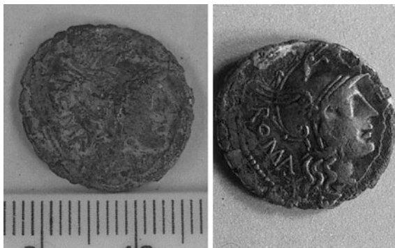
Fig. 6.73 Laser cleaning of roman coins. The photograph on the right reveals the inscripture after laser decontamination [85]
