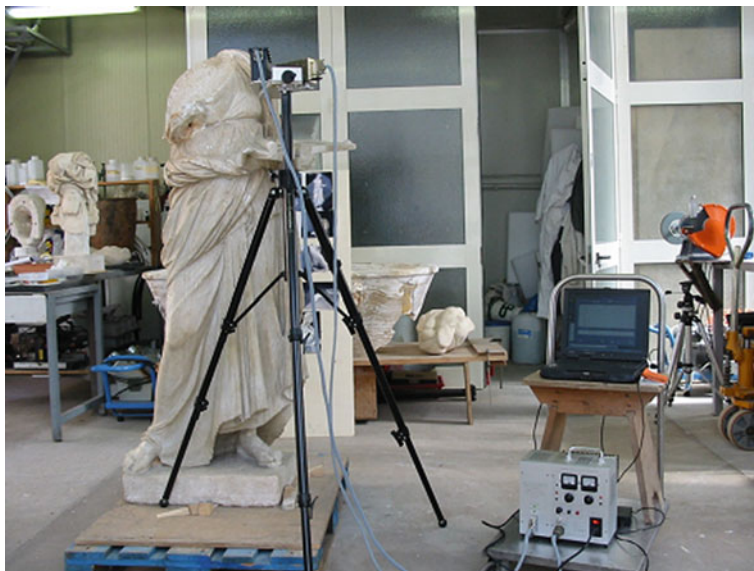
Fig. 4.7 Low energy XRF apparatus at work in the mapping of the ancient roman statue “Fanciulla di Anzio” in Rome
