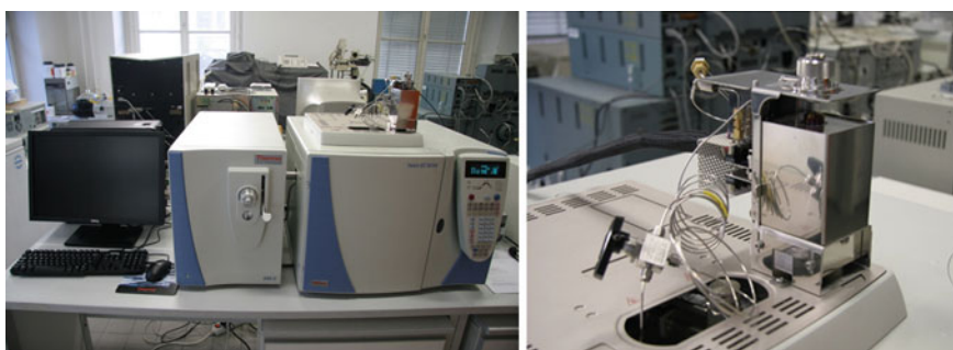
Fig. 5.38 FrontierLab-Thermo Ultra GC/MS, a Py-GC/MS equipment, b Pyrolyser unit
