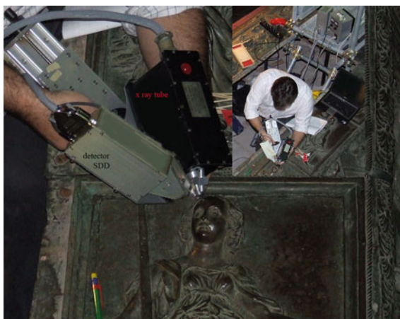
Fig. 6.33 Non-invasive measurements with a portable EDXRF on the funeral monument of Pope Sixtus IV
