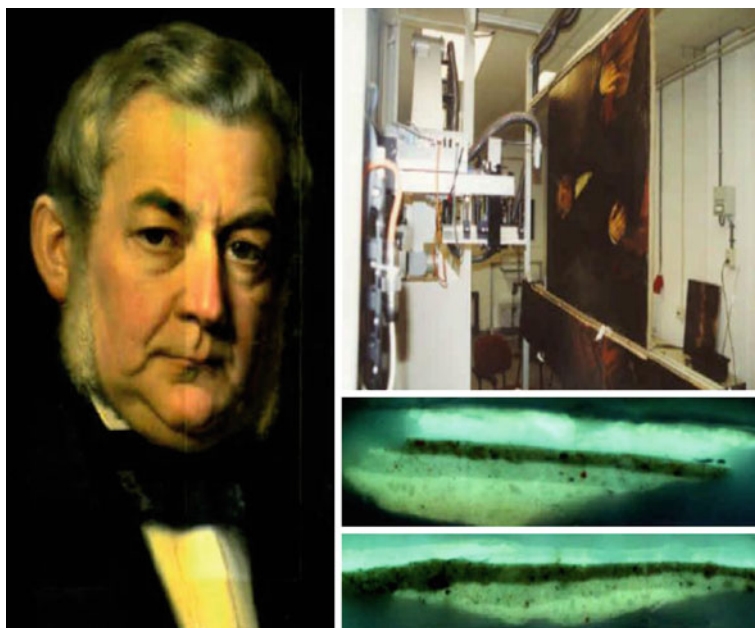
Fig. 6.74 Laser decontamination of a portrait by J.H. Neuman. A distinct contrast difference may be observed between the contaminated original painting ( left ) and the laser decontaminated surface ( right ) of the portrait's face. A cross-section micrograph shows the difference between the original ( top image ) and the laser treated surface ( bottom image ) [86]
