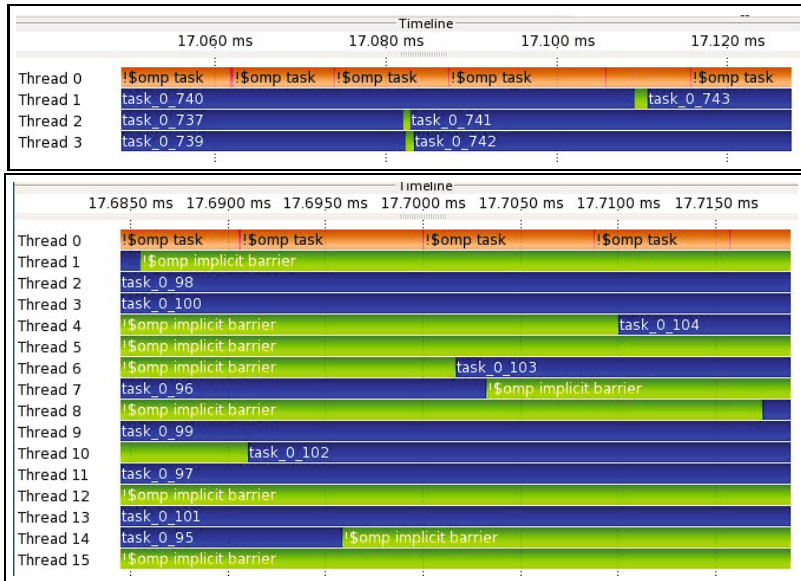
Fig. 7. Vampir screenshot illustrating how a task-creation bottleneck can be detected. Both timelines show the same program where a single thread creates tasks for all other threads. Top: With four threads every worker thread is busy, executing tasks. Bottom: With 16 Threads some threads are idle and wait for tasks from the master thread.
