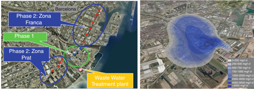
Fig. 8 Left: Injection wells of the full hydraulic barrier (phases I and II) and location of the WWTP. Right: Reduction in chloride content in the aquifer between 2007 and 2009, indicating the movement of water injected by the hydraulic barrier in Phase I
