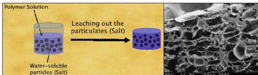
Fig. 2 Schematic of particle leaching fabrication method. The polymer solution is placed in a mold with some sort of porogen (i.e. salt) and then a scaffold is formed. The porogen is then washed out of the scaffold, leaving a network of interconnected pores [31] ( left ). SEM images of porous ceramic scaffold fabricated through particle leaching method through dissolution of the porogen [32] ( right )
