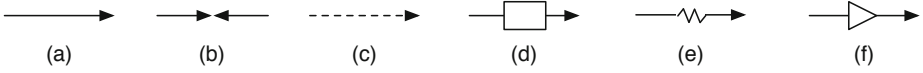
Fig. 1. Common channel notations: (a) Synchronous (b) Synchronous Drain (c) Lossy Synchronous (d) FIFO-1 (e) Filter (f) Transform
