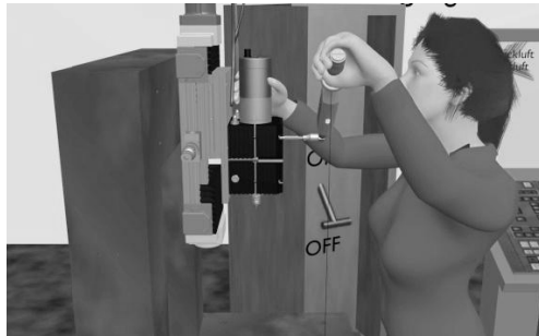
Fig. 6. Screenshot of Avatar Video Guidance shown on a display in the field of view of the operator
