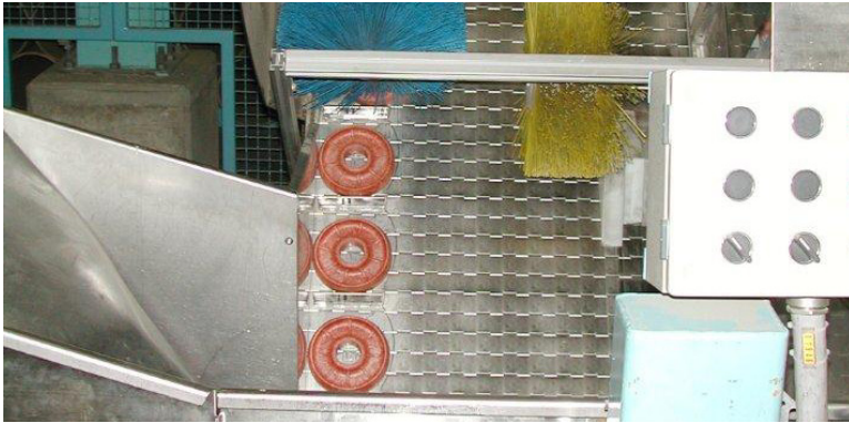
Fig. 4. Cleaning of used core plugs at the paper mill company
