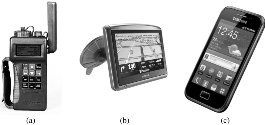
Fig. 3. Historical development of GPS receivers, from bulky positioning devices (a) over smart navigation devices with map functions (b) to small modules integrated into smart phones (c)
