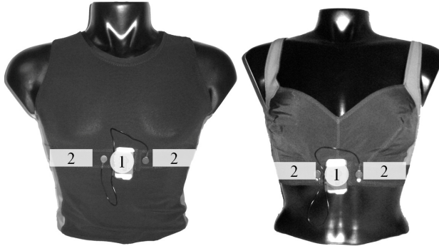
Fig. 1. Male vest garment (left) and the female bra garment (right). Within the images 1 is the Shimmer device placed within a pocket on the front of the garment. 2 depicts the location of the TE.
