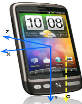
(a) Orientations of accelerometer
