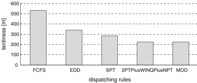
Fig. 2 Simulation results in mean tardiness with 30 replications; 99 % confidence level to MOD (paired-t confidence interval)
