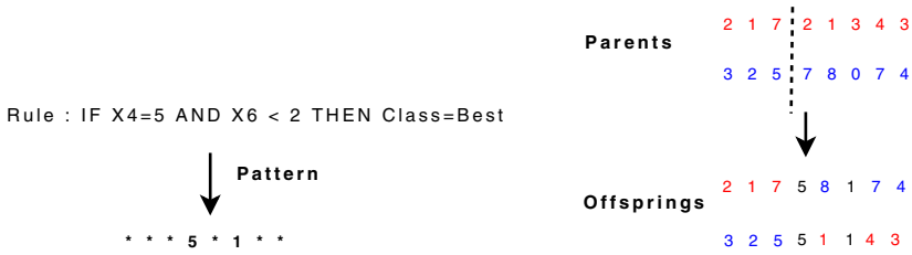
Fig. 1.34 Crossover operator using the induced rule as a pattern. For instance, the extracted pattern (...5.1..) is included into the offsprings.
