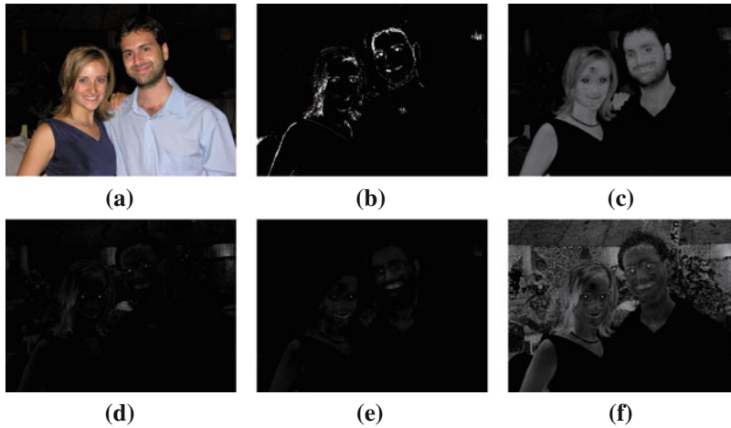
Fig. 12.5 Examples of redness maps: a original image; b–f redness maps obtained with Eqs. (12.1)–(12.5), respectively
