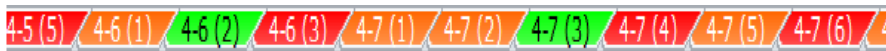
Fig. 7. Staining tab code color following the readiness of the deliverable. Each tab represents the deliverable of a certain process with its rank. For example 4-6 (1) is the first output deliverable of the subprocess 4-6 (clause 6 of part 4 of ISO26262).
