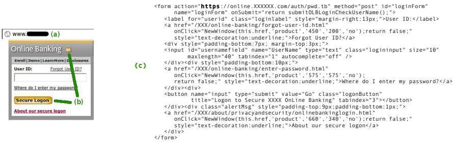
Fig. 1. Screenshot of the login box on the home page of a bank. Notice (a) that the page is served on HTTP, (b) the graphics suggesting a secure login process, and (c) the underlying HTML code, which sends data on HTTPS, that is, as long as a MITM attack does not modify it.
