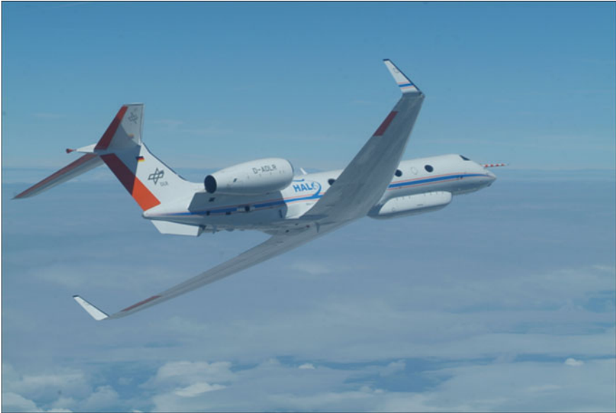
Fig. 37.7 HALO during belly pod and ventral fin flight tests photographed from the FALCON, which chased HALO to observe the behavior of the modifications. The belly pod is below the fuselage in front of the wings. The ventral fin is below the tail of the fuselage. Both structures can be removed
