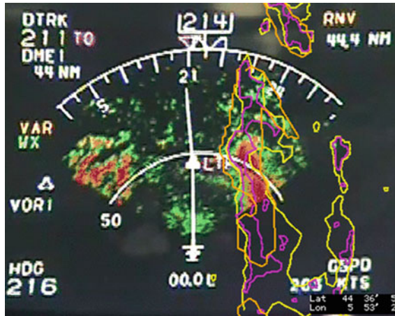
Fig. 39.1 Snapshot of a video of the on-board weather radar image from the French research aircraft SAFIRE ATR-42 close to Grenoble for 14:05 UTC on August 19, 2008 with subsequently superimposed weather object contours from the ground system. The colored shading represents the radar returns from precipitation or ground clutter with green indicating light , orange moderate , and red strong radar returns. Orange contours indicate Cb-TRAM objects; yellow and pink contours indicate heavy precipitation cells for two different intensities representing moderate and severe precipitation, respectively. (Figure adapted from Taffermer et al. (2010), © American Meteorological Society)
