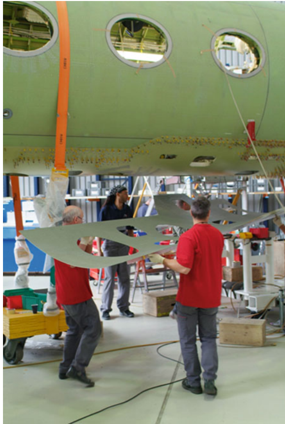
Fig. 37.1 HALO during modification at RUAG Aerospace. Due to the number of apertures, the fuselage structure must be triple-reinforced around the openings to retain its original stiffness
