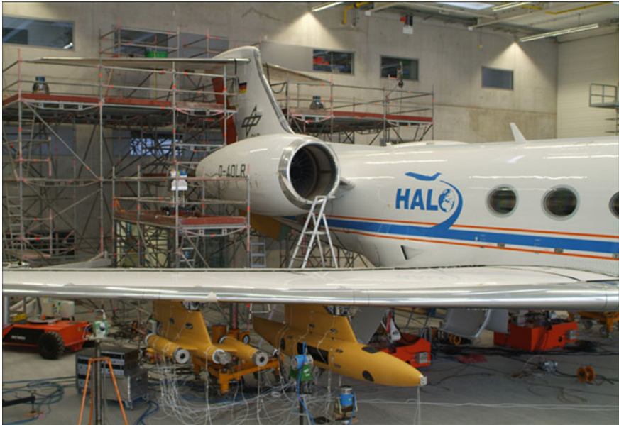
Fig. 37.5 HALO jacked-up and with scaffolding during ground vibration tests in spring 2009. The yellow installations below the aircraft wing are a carrier for particle measurement probes ( left ) and the under-wing instrumentation pod ( right )
