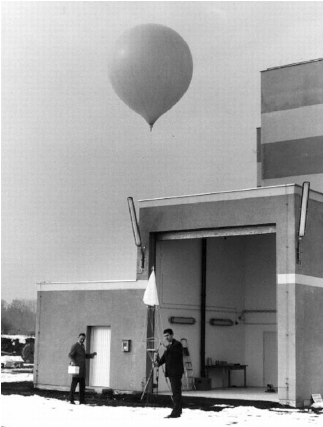
Fig. 19.1 Preparation of a radiosonde launch in front of the balloon hall of the institute (picture taken at IPA about 1974)
