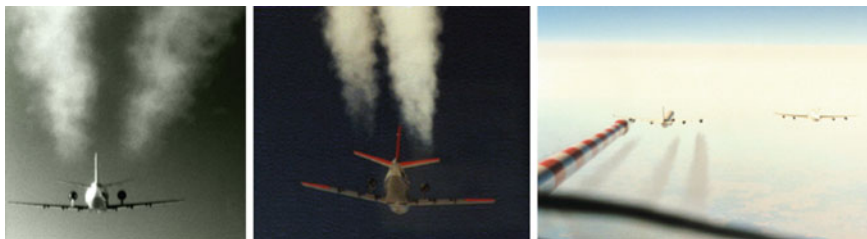
Fig. 15.1 Contrail formation at threshold conditions. Left Contrail formation for fuels of different sulfur content, FSC (FSC for left/right engine in \mu\text{g/g} , respectively: 1.6/245, Busen and Schumann (1995)]. Center Same for 170/5500 (Schumann et al. 1996). Right Two aircraft at comparable flight conditions with different overall propulsion efficiency \eta [ left < 0.24 , right > 0.28 , Schumann et al. (2000)]. (Photos: R. Busen, P. Thomas, U. Schumann, DLR)
