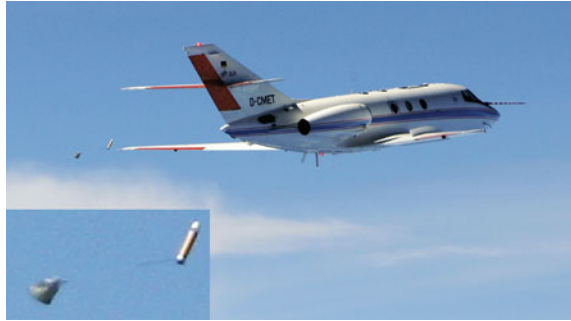
Fig. 19.4 Dropsonde release from the Falcon aircraft for measurements during the T-PARC project over the western North Pacific in September 2008. Shortly after launch the parachute is just being inflated, as seen in the enlarged cut-out. Picture with courtesy of The Yomiuri Shimbun
