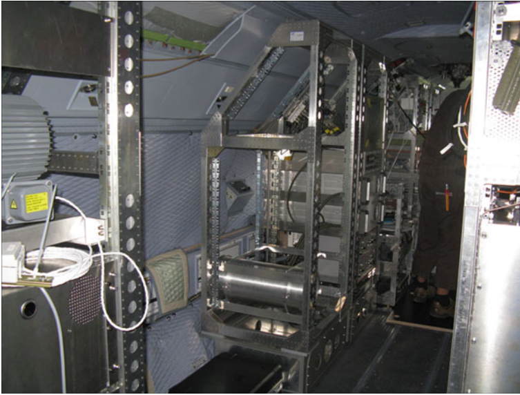
Fig. 37.4 Scientific instruments in the cabin are usually integrated into standard racks mounted between seat rails on the cabin floor and attached to additional rails above the cabin windows
