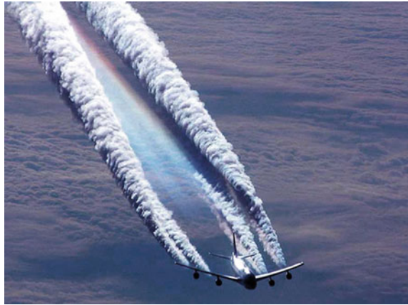
Fig. 33.1 Photograph showing a contrail produced from a Boeing B747 with four engines. Two contrail formation modes are visible: exhaust contrails becoming visible shortly behind the engines, and an aerodynamically produced contrail. The latter is the faint iridescent ice sheet in the middle between the thick exhaust contrails. Copyright Josef P. Willems
