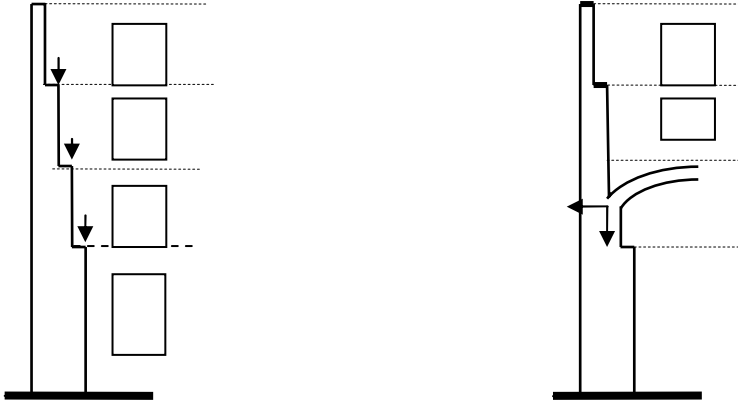
Figs. 7.22 and 7.23. Facade walls. Opposing and concurring actions of floor loads, wall weights, and vault thrusts
