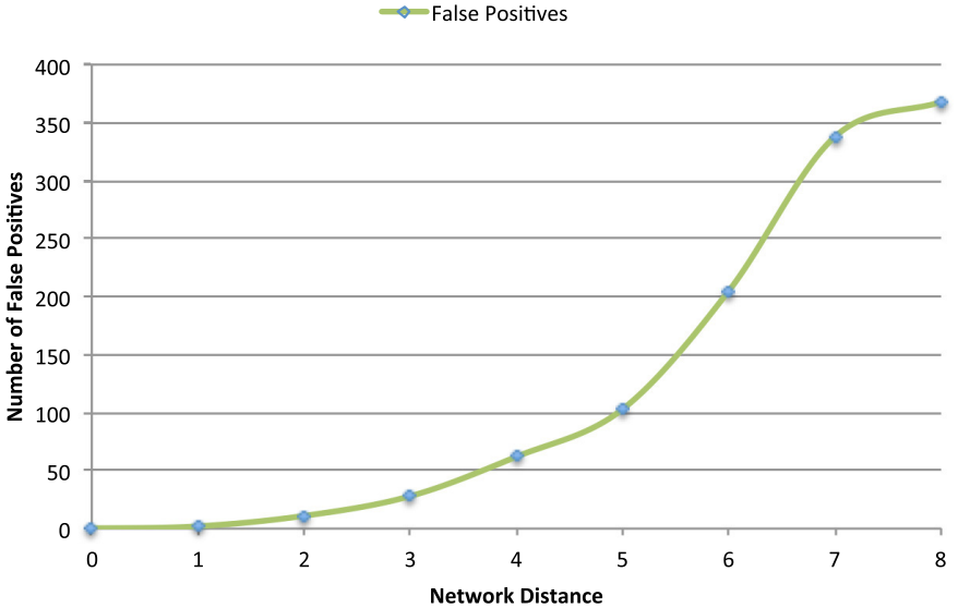
Fig. 4.10 The number of false positive responses in 100,000 random provenance queries checking if an edge exists between two network vertices using the matrix filter sketch of a host. The provenance is of a synthetic workload, consisting of a sequence of network connections through consecutive hosts.
