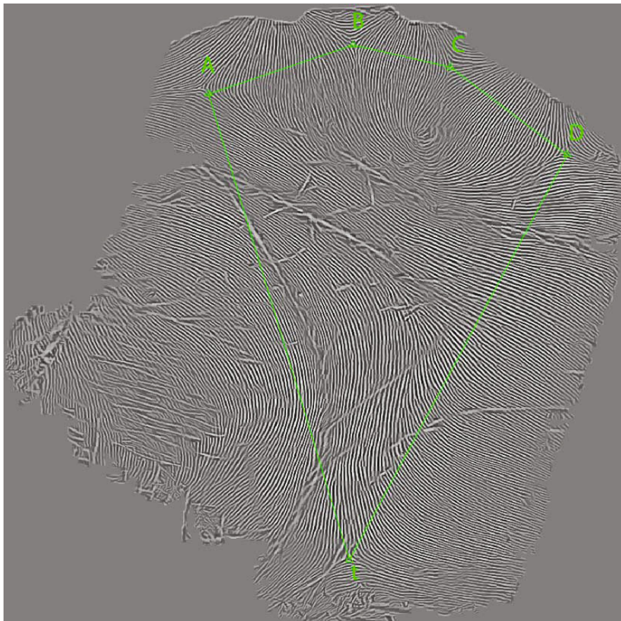
Fig. 4 Singular points of the palmprint located using two stage algorithm taking advantage of improved Poincare index and Gauss-Hermite moments
