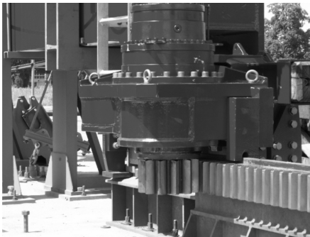
Fig. 9.3. Rack travel system
