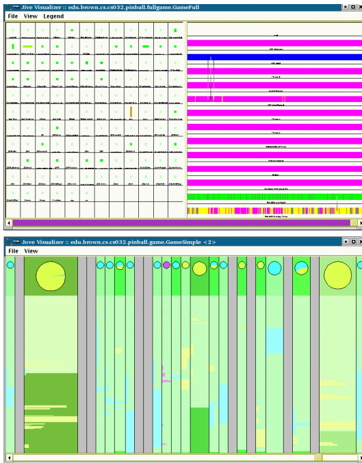
Fig. 1. Jive and Jove dynamic visualizations. The first window shows Jive with the lefthand panel shows execution time and allocations by class or package; the right hand panel shows thread activity and interactions. The second window shows Jove which provides line-level usage information for the classes in a system.
