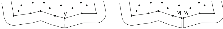
Fig. 6 The bottom part of an ( \alpha, \delta )-sleeve, the lowest vertex v of the \alpha -shape (left), and the conversion of the sleeve to a simple polygon (right)
