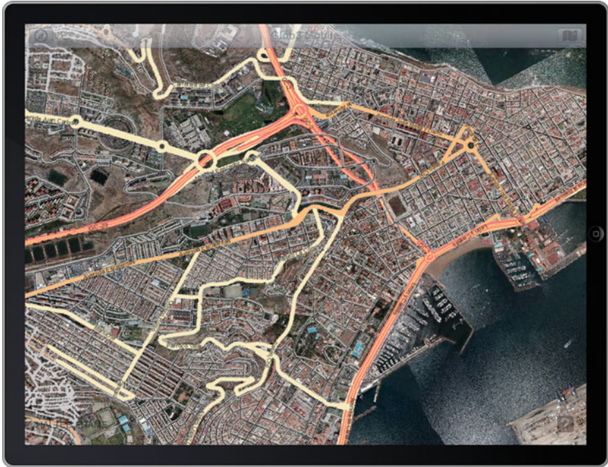
Fig. 10 Displaying a transparent texture (street map of a city) merged with an aerial photo
