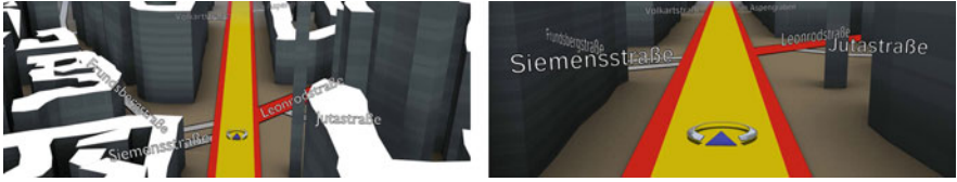
Fig. 3 Baseline: drawing labels over the 3D world in bird's eye with SS ( left ) and snail view with WS labeling ( right )
