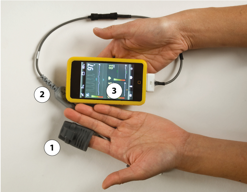
Fig. 2. The Phone Oximeter (mobile phone pulse oximeter) application. 1) Soft finger probe; 2) Nonin Xpod OEM pulse oximeter module; 3) iPod Touch with raw PPG waveform, SpO 2 and HR trend display.
