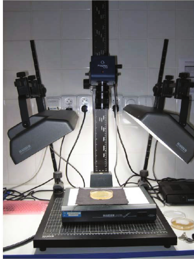
Fig. 1. General-purpose imaging setup used with the proposed colony counter
