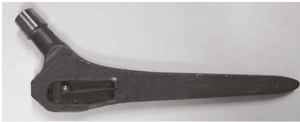
Fig. 2. Total hip stem with one oscillator placed in the proximal part
