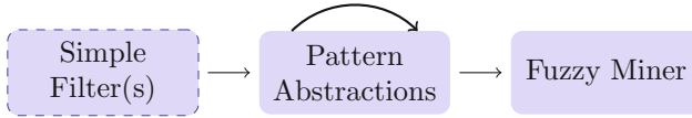
Fig. 3. The chaining of plugins that enables the discovery of hierarchical process models
