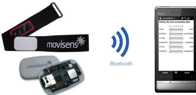
Fig. 5. Integrated measurement system for assessment of stress
