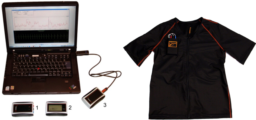
Fig. 1. Night time HR measurement hardware. Measurement unit marked as 1, display unit as 2, and network coordinator as 3.
