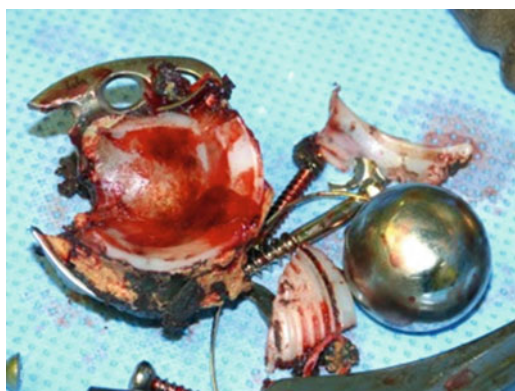
Fig. 13.3 Wear and destruction of a polyethylene inlay and a revision cup as a possible complication of edge loading
