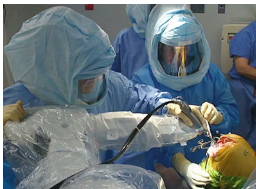
■ Fig. 12.3 Intraoperative set-up of the MAKO system during a robotic-assisted unicompartamental knee arthroplasty. (By courtesy of MAKO Surgical Corp.)
