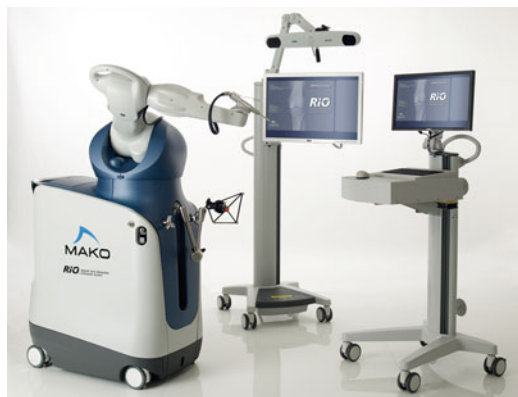
■ Fig. 12.1 The »Robotic Arm Interactive Orthopedic System« (RIO) as an example of a surgeon-guided robotic system. (By courtesy of MAKO Surgical Corp.)
