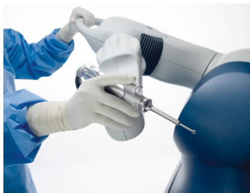
■ Fig. 12.2 The high-frequency burr is equipped at the distal end of the robot. (By courtesy of MAKO Surgical Corp.)
