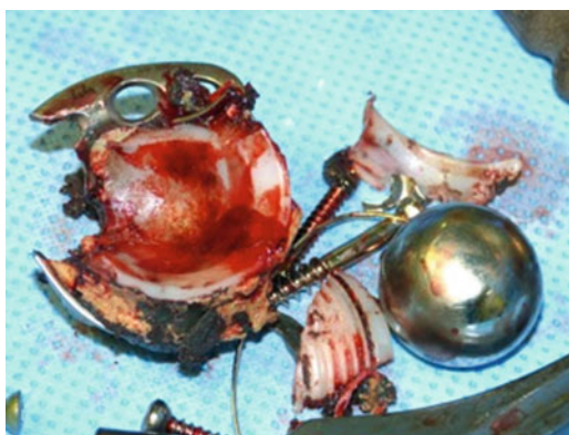
Fig. 13.3 Wear and destruction of a polyethylene inlay and a revision cup as a possible complication of edge loading
