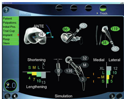
Fig. 14.1 The simulation screen allows one to change the values of the CCD angle as well as the ante- or retroversion; it displays the changes in the values for antetorsion of the femoral neck and the range of motion. (By courtesy of B. Braun, Aesculap)
