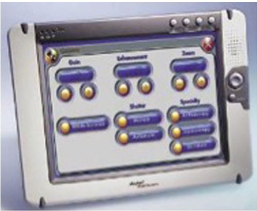
Fig. 19.5 Touch-screen controls are stationed at the non-sterile area to be operated by nursing/assisting staff. (From Hübner et al. 2012)
