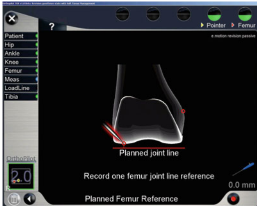
■ Fig. 9.1 The screen asks the surgeon to palpate the reference point on the femur from which he has calculated his future joint line
