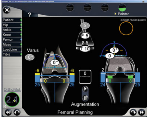
■ Fig. 9.3 The planning screen. On the left side the situation in extension is simulated, on the right side the situation in flexion. In the middle (top part) , the component sizes are shown (in this case a femur of size 5 with a distal thickness of 8.5 mm and a tibial component with a total thickness of 10 mm). Below, the component inside the square is the distance from the planned distal joint line. The screen is shown after measuring the extension gap ( left side ) and flexion gap ( right side ). The values are indicated in blue numbers and columns . On top of the blue columns , the amount of bone that has to be resected is indicated in white (right side) or the missing bone is indicated in yellow (left side) as a trigger for necessary augments
