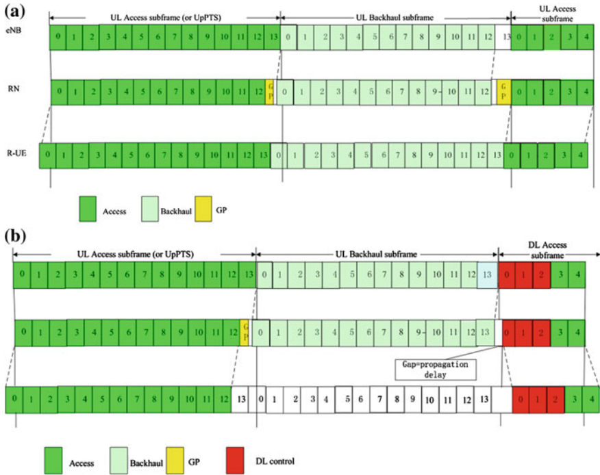
Fig. 4.6 a Example for subframe relationship when eNB-RN distance is between 6 and 15 km, and UL backhaul subframe is followed by an UL access subframe. b Example for subframe relationship when eNB-RN distance is between 6 and 15 km, and UL backhaul subframe is followed by a DL access subframe
