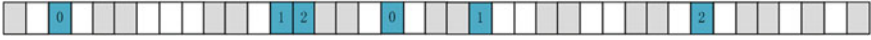
Fig. 4.23 Association of subframe number and HARQ process ID (numbers referred to the subframe numbering)
