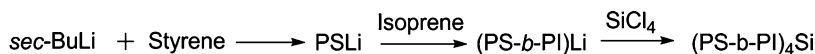
Synthesis of Star Polymers, Fig. 21 Synthesis of star-block copolymers of PS and PI
