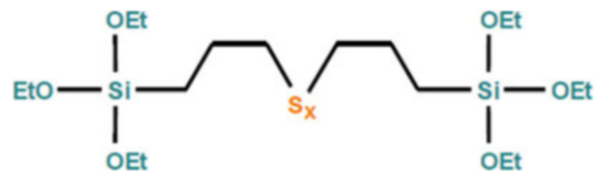
Silica Reinforcement, Fig. 3 Commonly used silane for tire tread applications ( x = 3.7 )
