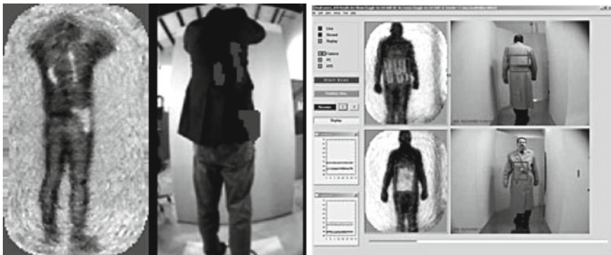
Fig. 19.3 (Left) Still frames from 10 fps passive mm-wave video imagery (MMW and visible with privacy overlay algorithm) from the Millivision Portal 350 system. (Right) The user interface of the Millivision Walk-by 350 system. [64]
