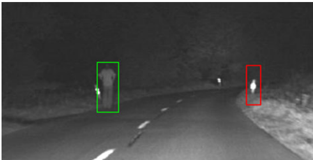
Fig. 1 An example of a true positive (green) and a false positive (red) detection of the cascaded classifier.
