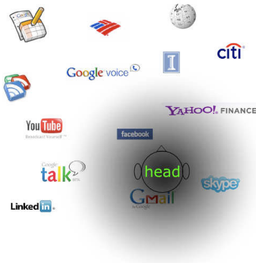
Fig. 1. Consuming multiple audio web streams in 3D audio space. The “head” indicates the user in the virtual audio space. The gradient shading shows that closer web streams are relatively louder.
