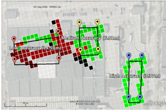
Fig. 2. Visual overlay for a shopping mall as a colored map with scale from bright green (high accuracy) over red to black (low accuracy)
