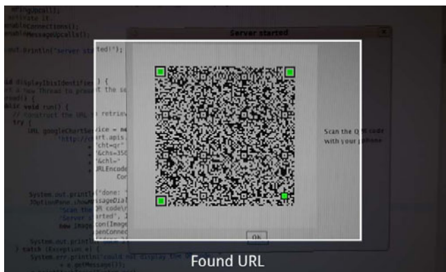
Fig. 4. A screenshot of the resource manager collecting the address of a remote resource. From now on this resource is known to the smartphone and will be used by any application that uses Cuckoo for computation offloading.
