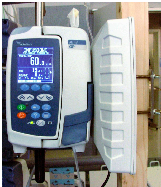
Fig. 1 868MHz passive RFID transmitter – Infusion pump test a right face test in contact.
