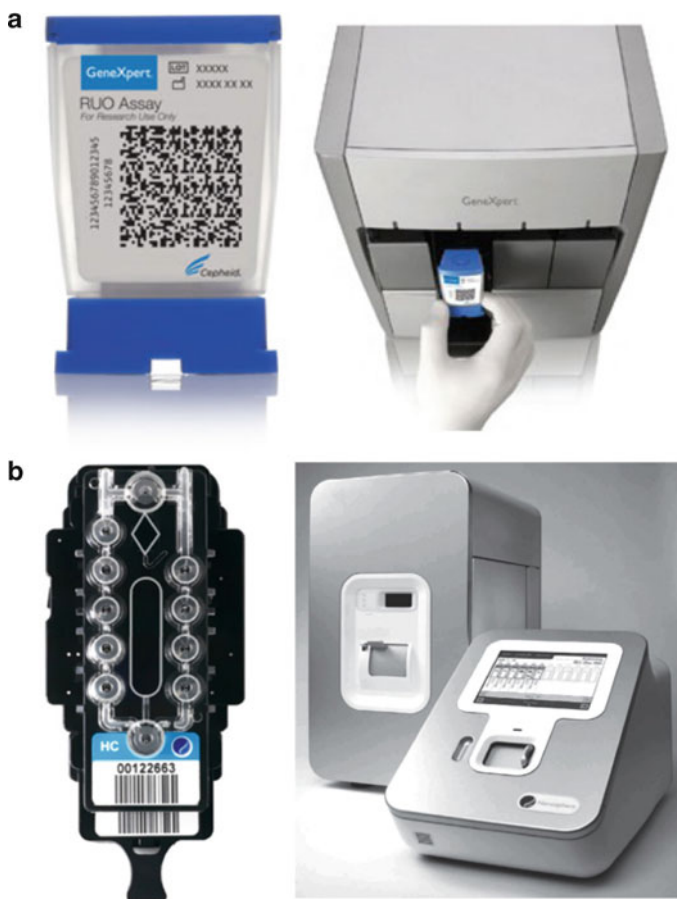
Fig. 1.5 (a) Cepheid's GeneXpert test platform ( right ) integrates sample processing and PCR in a disposable plastic cartridge ( left ) containing reagents for cell lysis, nucleic acid extraction, amplification and amplicon detection. This system has been used to detect drug-resistant tuberculosis cases (Taken from www.cepheid.com with permission from Cepheid, Inc.) (b) Nanosphere Verigene system. Picture of a Nanosphere cartridge with loaded reagent wells ( left ). Picture of Verigene readers with touch-screen control panels ( right ) (Taken from www.nanosphere.us with permission from Nanosphere, Inc.)
