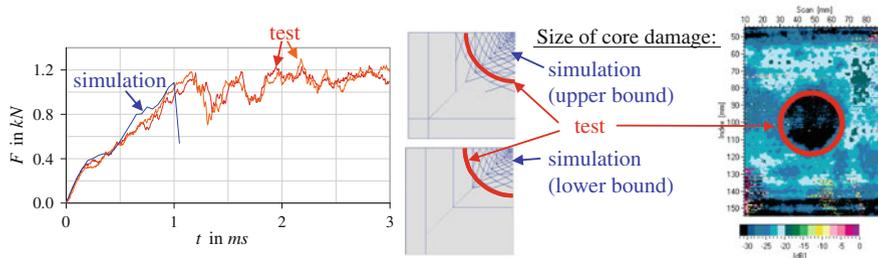
**Fig. 13.4** Simulation results: Force-time history and core damage compared with test results
