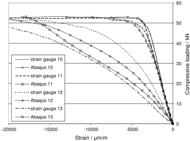
**Fig. 13.7** Comparison between simulation results and test results: strains in loading direction in the vicinity of the 4 J impact versus compressive loading of the panel. Strain gauges are located abreast the impact damage with a distance between 7.5 mm (strain gauge 13) and 31.5 mm (strain gauge 10) from the damage centre [20]
