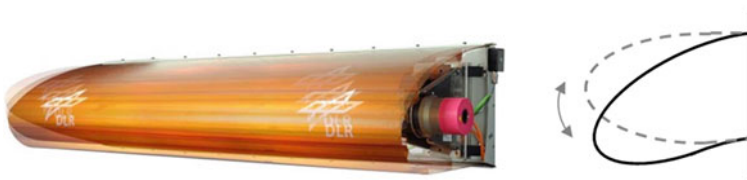
Fig. 17.9 Morphing leading edge high lift device
