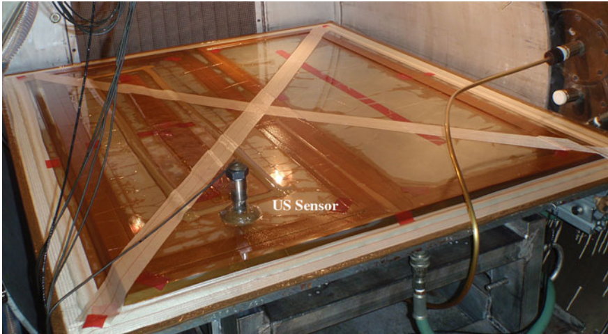
Fig. 29.8 Manufacturing of coupon panels
