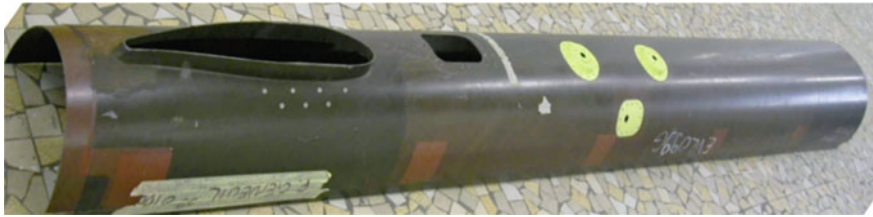
Fig. 37.10 Tailboom (half-shell) of Eurocopter EC 135
