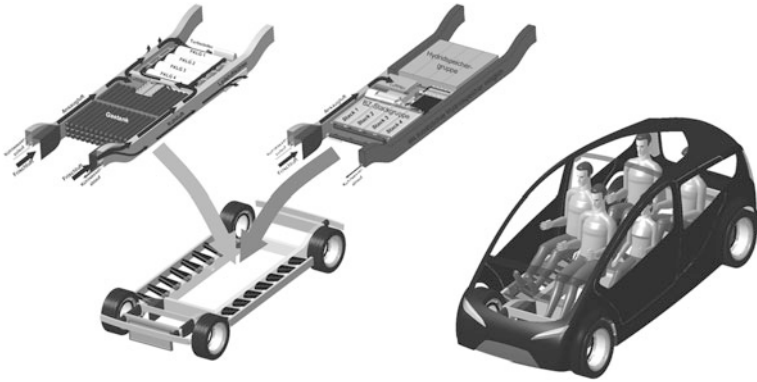
Fig. 22.1 Vehicle concept with intrusion-resistant containment (DLR courtesy)
