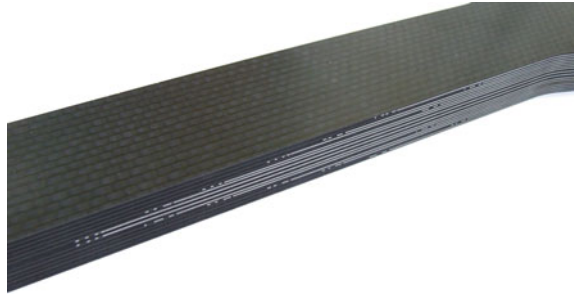
Fig. 19.10 Transition region (CFRP/steel, resin infusion)
