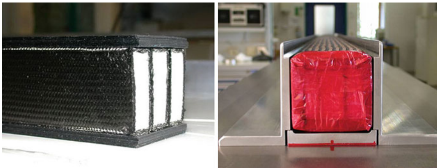
Fig. 28.8 Manufacture of the spar with prepreg belts ( left ); spar with final wrapping in the tool ( right )
