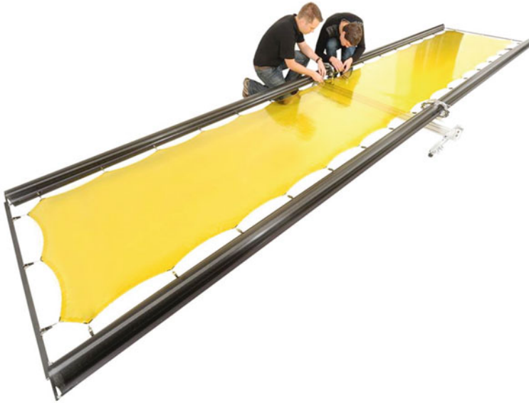
Fig. 18.6 1:3 sub scale model of a deployable SAR antenna (model size 6 × 1.4 m)
