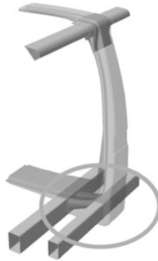
Fig. 22.6 Functional area of B-rib: crash cone element
