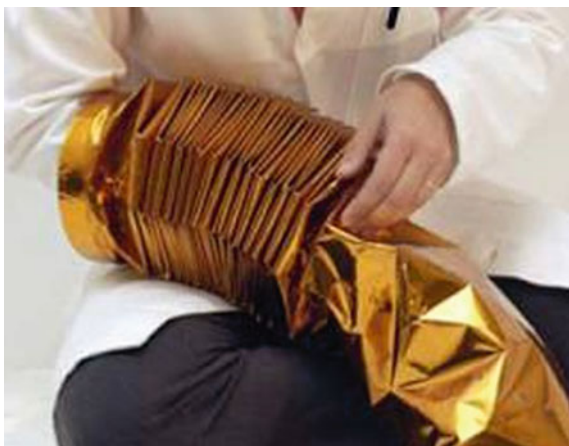
Fig. 18.4 Inflatable boom during folding (Courtesy of ASTRUM)
