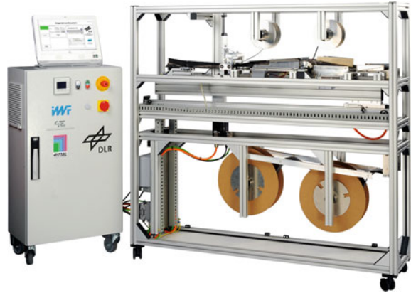
Fig. 25.3 Fully automated continuous preforming machine for profiles with variable web height
