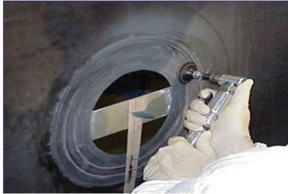
Fig. 23.1 Manual scarfing by angular grinding [7]
