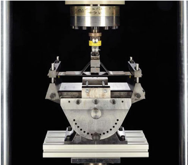
Fig. 16.7 Stringer Pull-off device with stringer skin specimen
