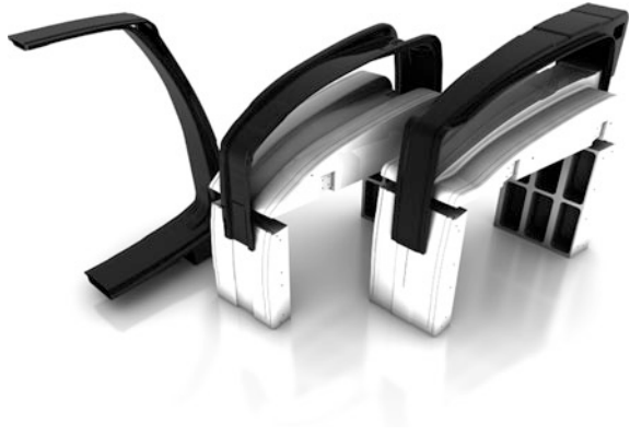
Fig. 22.10 Prototype B-rib (half, rendering) and autoclave tool concept
