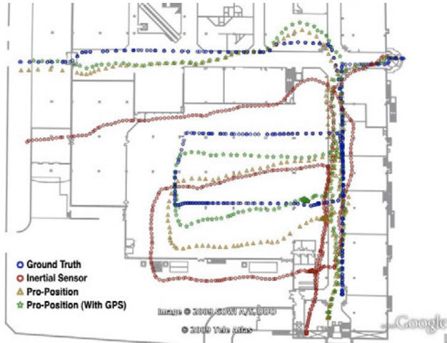
Fig. 1. Results from inertial sensor measurements, Pro-Position with and without GPS together with the ground truth path in a shopping mall
