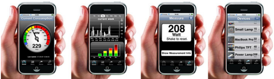
Fig. 2. The UI (left to right): Consumption view, history view, measurement view, and device inventory view
